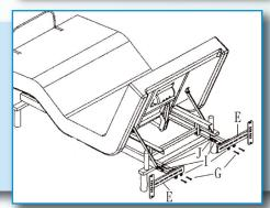
**iV.** When headboard brackets are assembled, make sure there is a space of 1.5 (38.1 mm) to 2 inches (50.8 mm) between the edge of the bed base and the headboard brackets.
