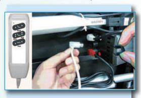
**Step 2-1** Take out the Pairing Cable. The 90° plug head with the longer part of cable is for connecting the black control box. Straight plug head with shorter part of cable is for connecting the handset remote.
