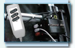
**Step 1-2** Take out the wire cap and remove the plug of the handset from the control box. (Same steps for the second bed frame)
