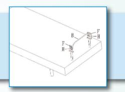
**NOTE:** Use **ONLY** the allen wrench to fasten the retainer bolts. **DO NOT** use a power screwdriver as it may over tighten the bolts. Mattress retainer hardware must **NOT** be over tightened.
